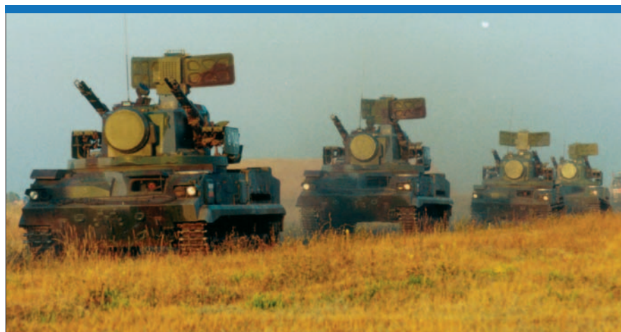
Up to six 34-tonne Ulyanovsk Tunguska-M1 systems provide a complete combat unit in conjunction with a Tar 9C18M1 long range radar and battery command post, all mounted on the same tracked chassis. (Armada archives)
