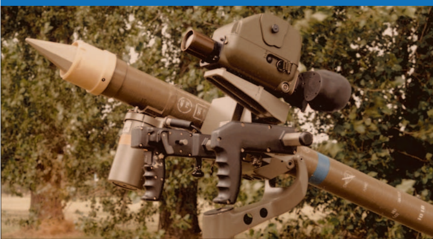
One of the most popular man-portable Sams is the MBDA Mistral, shown here with a Thales MITS-2 thermal imaging sight, allowing long-range target detection. (Thales)
