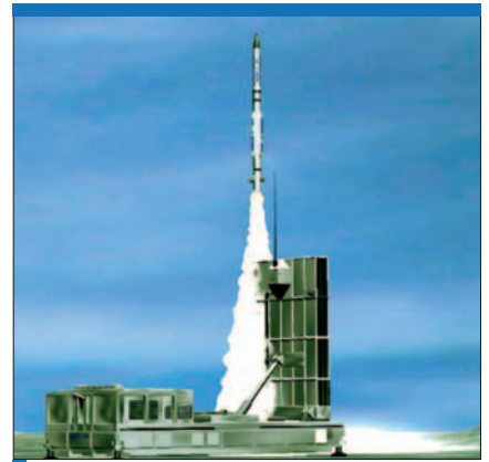
As MBDA has done with the Mica, BGT and Eads-LFK developed a VL launch system using the air-to-air Iris-T, which was unveiled at the ILA 2002 exhibition. (BGT)
