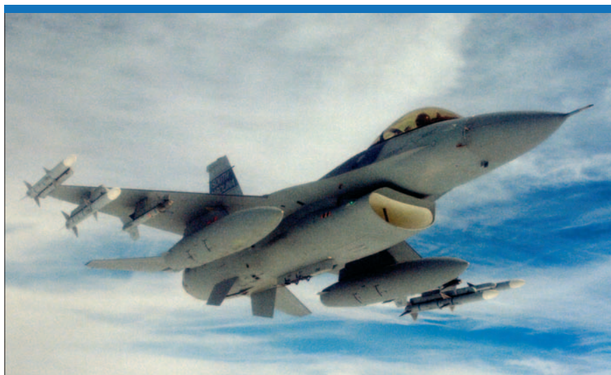
This South Carolina Air National Guard Lockheed Martin F-16C is armed for the air defence role, with four Raytheon AIM-120s and two AIM-9s. (Lockheed Martin)
