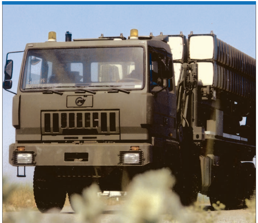
The Eurosam Samp-T is an easily deployed launch unit that is based on standard army trucks, more specifically the French Renault TRM and the Italian Astra/Iveco, as illustrated here. (MBDA)
