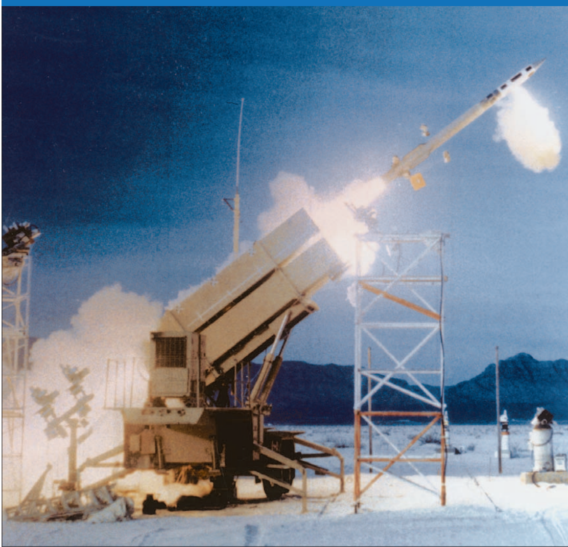
The Lockheed Martin Pac-3 missile is to be used by both Patriot and Meads. Although relatively small, it provides enhanced capability against ballistic missiles. (Lockheed Martin)
