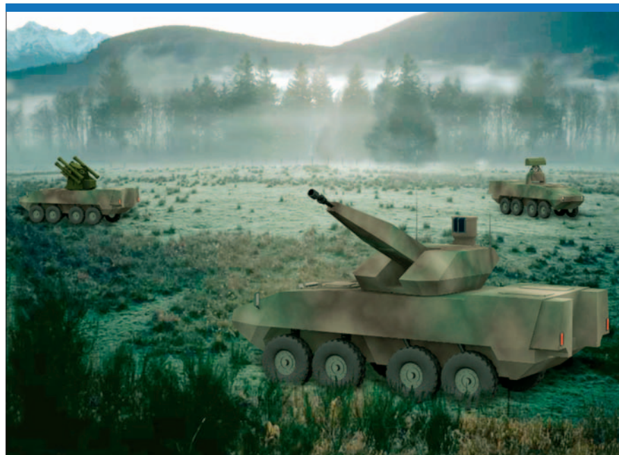
Using the Skyshield 35 as a foundation, Oerlikon is currently working on the concept of a self-propelled battlefield air defence system using the revolver-Ahead combination with a tactical command post equipped with the company's new 25 to 50 km-range X-Tar 3D radar (at right in background). The aim is to make the units C-130 transportable. (Oerlikon Contraves)
