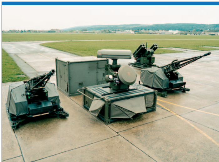
While a Skyshield 35 fire control system can control two guns, or two guns and a missile launcher, it could handle up to four guns; however, such a combination would simply result in an overkill, such is the effectiveness of the 35/1000 firing the Ahead. (Oerlikon Contraves)
