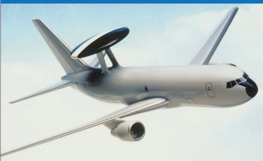
The Boeing E-767, based on the B767-200ER, replaces the E-3 Awacs, the B707 line having closed in 1991. So far only Japan has ordered this aircraft. (Boeing)
