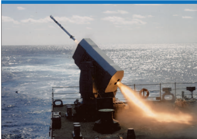
The Ram (Rolling Airframe Missile) is a joint US-German development by Raytheon and the Ramsys consortium. It is shown here being fired from a 21-cell launcher. (Raytheon)
