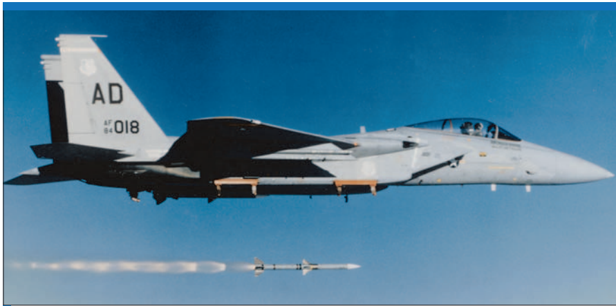
Test firing of a Raytheon Aim-120 Amraam (Advanced Medium-Range Air-Air Missile) from a Boeing F-15C. The Amraam entered service in 1991, and is also used as a surface-air missile. (Raytheon)
